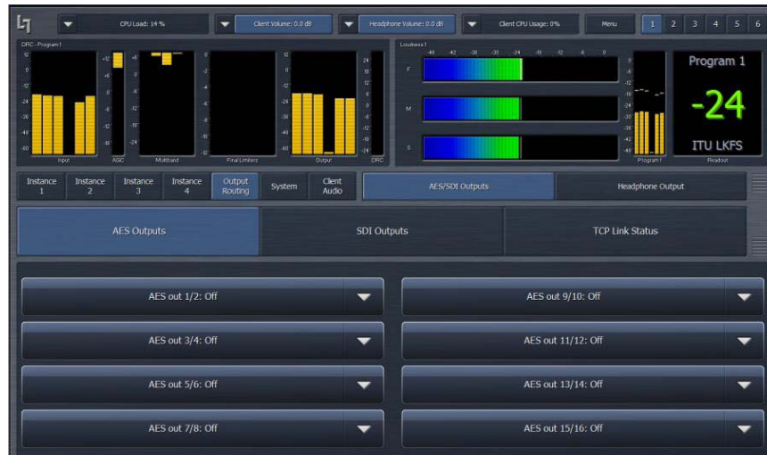
Figure 1-9 The AES and SDI Outputs tabs allow source selection for each physical output
